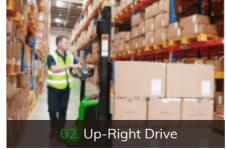
Easily maneuvered with the handle in the vertical position by pressing the turtle-speed button.
